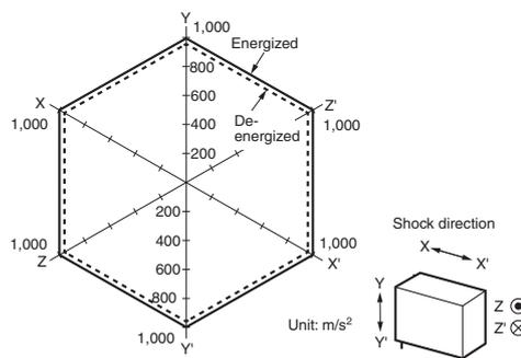
Conditions: Shock is applied in ±X, ±Y, and ±Z directions three times each with and without energizing the Relays to check the number of contact malfunctions.
